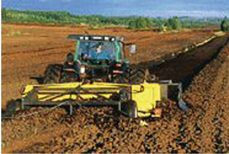
Fig. 2.3 This machine cuts and macerates the peat and then sends it along the extended arm which deposits it in rows. The peat is cut into blocks by the discs as the equipment moves forward
