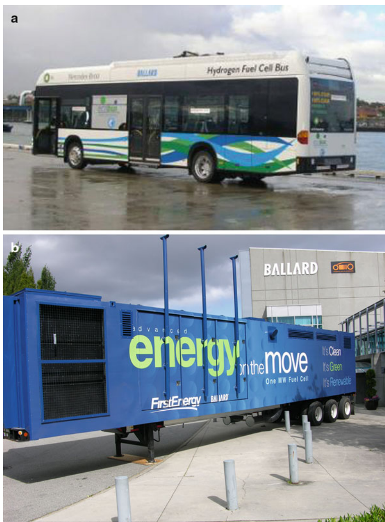
Fig. 9.15 (a) The Ballard H_2 fuel cell-powered bus and (b) the FirstEnergy fuel cell unit (Ballard Power)
