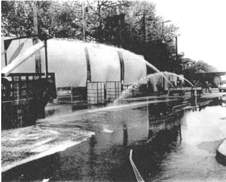
Fig. B.6 Effect of high molecular weight polyethylene oxide) in increasing water flow through fire hoses. Hoses had been adjusted to throw water the same distance and then 30 ppm of polyethylene oxide) were injected into the hose on the left
