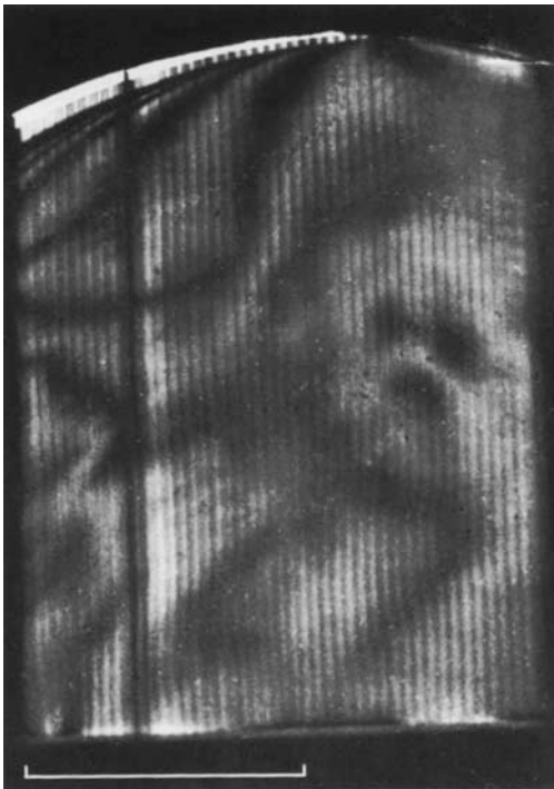
Fig. II.3. Moiré topography of the silicon interferometer. The vertical lines are due to the fact that the pattern is recorded in strips
