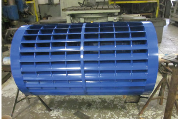
Fig. 6.26 The runner of a crossflow turbine resembles a squirrel cage (courtesy of Canyon Industries)
