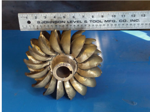
Fig. 6.18 This small (22 cm diameter) runner for a Pelton turbine can be used to supply over 10 kW of power
