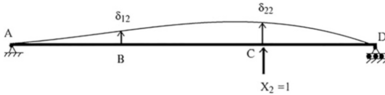
Fig. E9.3d Deflected shape due to X_2 = 1
