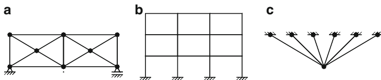
Fig. 1.4 Some simple structures. (a) A planar truss. (b) A planar frame. (c) A simple planar truss
