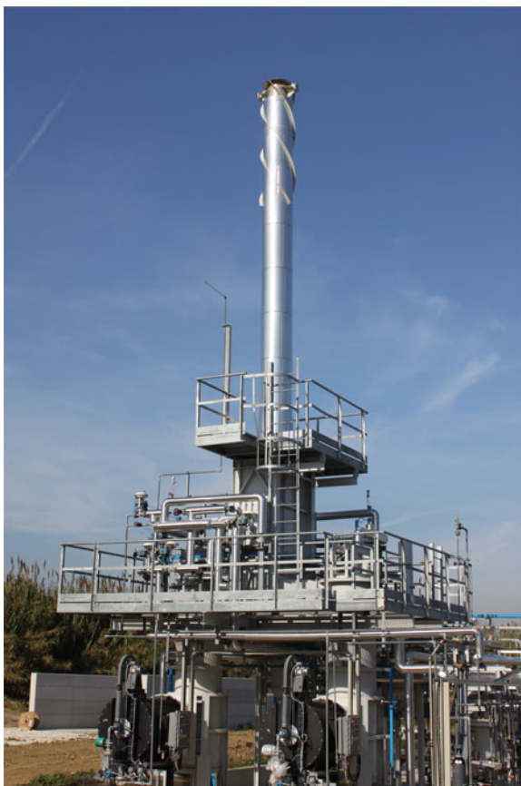
Fig. 1.4 20 Nm 3 /h of pure H 2 capacity RMM plant (Courtesy from Tecnimont KT)
